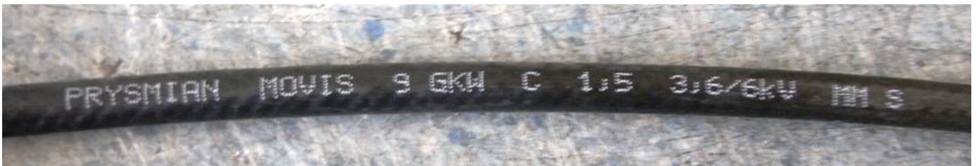
CABLE MARKING : PRYSMIAN MOVIS 9 GKW C 1,5 3,6/6KV MM S
