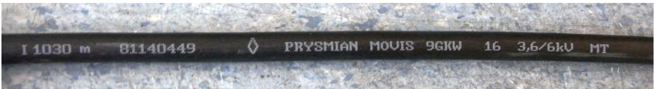
CABLE MARKING : I meter marking 81140449 PRYSMIAN MOVIS 9GKW 16 3,6/6KV MT
